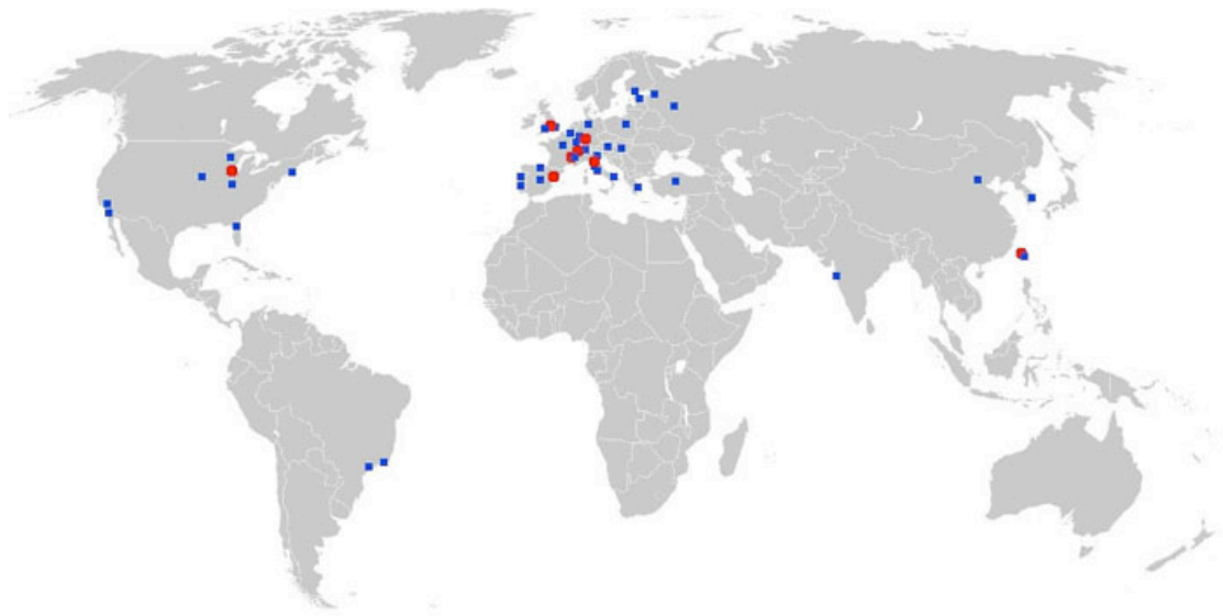
Figure 3.15: A map showing the geographical distribution of CMS Tier 1 (red dots) and Tier 2 (blue dots) data centres. Reproduced from [9].
